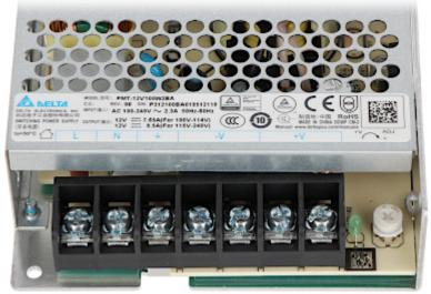
L - Live wire (230V) N - Neutral wire GND - Grounding -V - DC "-" output +V - DC "+" output ADJ - Output voltage adjustment Top view:
