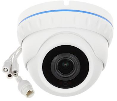
IP camera with efficient H.264 / H.265 image compression algorithm for clear and smooth video streaming at maximal resolution of 2592 x 1944 (5.0 MPx). The used motozoom lens with 2.7 ... 13.5 mm focal length allows to remote view angle adjustment.
