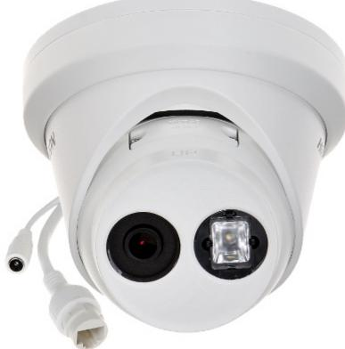
IP camera with efficient H.264 / H.265 image compression algorithm for clear and smooth video streaming at maximal resolution of 2688 x 1520 (4.0 MPx). PoE powering possibility, compatible with the 802.3af standard makes the device more universal and easier to
