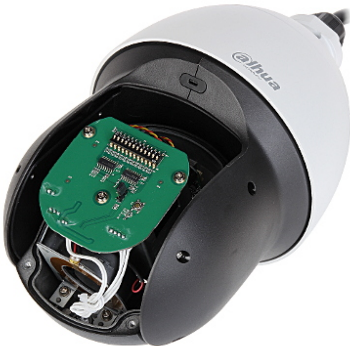
Bottom view (configuration switches visible):
