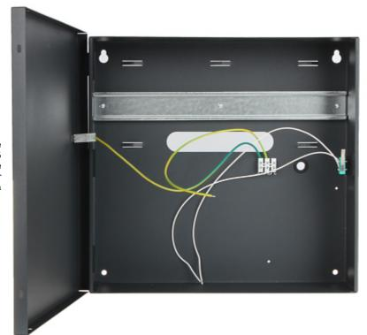
The ME-16 metal housing is dedicated for the installation of modules and devices of the RACS 5 system. The housing is equipped with a single mounting rail of the DIN TS-35 system and a tamper switch, and there is also space for a battery with a capacity of 17 Ah.
