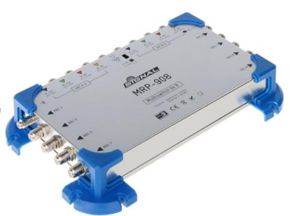
Attention! For unloaded outputs, use 75  $\Omega$  terminating resistors.
