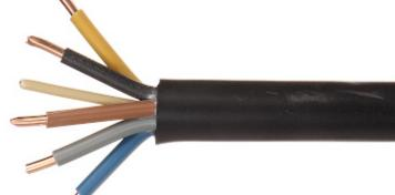
Electric cable for use in lines conducted in air, water, concrete, cable ducts and directly in the ground. The cable contains a protective conductor.
