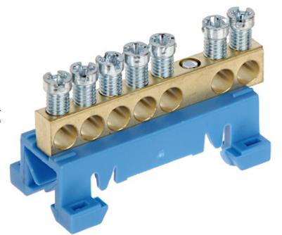
Distribution terminal block for using with modular distribution cabinets . Terminal block can be mounted on DIN TS35 rail crosswise.
