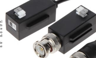
The PFM800B-4K is designed to video signal transmission via twisted-pair cable. The device adapts the impedance of coaxial cable  $75\Omega$  to the impedance of symmetrical line, ensuring transmission of video signal up to 400m (twisted-pair cable category 5) and eliminates asymmetric interferences.
