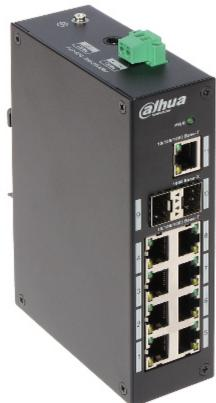
The DH-PFS3211-8GT Switch is an industrial type device enabling fluent network transmission at rates 10 / 100 / 1000 Mbps. Devices of this type can be used in installations realized in industrial facilities in harsh environmental conditions like high or low temperature. Attention! The SFP port requires the SFP module, which is available in our offer.
