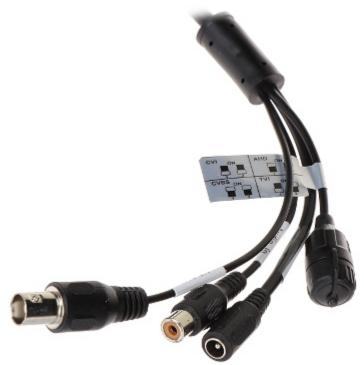
Standard changes are made using configuration switches:
