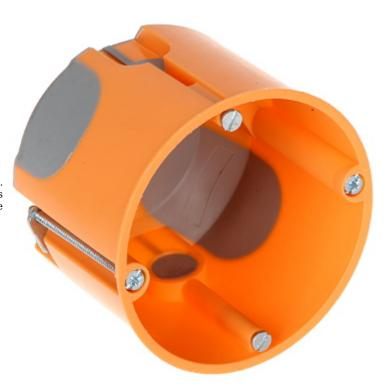
Flush electrical installation box, windproof with membranes. The box is intended for installation in hollow walls (plasterboard). Tightness of the box is ensured by flexible membranes.
