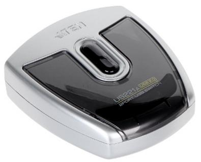
The US-221A USB switch allows to share a peripheral device (such as a printer or scanner) between 2 computers. The choice of the computer that has access to the device is made by a button located on the device casing.
