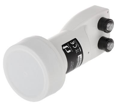
The KONW/WIDEBAND-INV is dedicated for installations working in the Wideband system, based on multiswitches. The LNB Wideband differs from standard quattro type LNBs in that it has two signal outputs (H + V) instead of four, so the installation based on one satellite requires only two satellite cables routed from LNB to the multiswitch.
