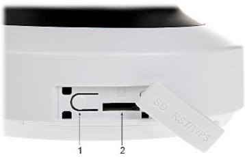
1. WPS/RESET button 2. Memory card slot Mounting side view:
