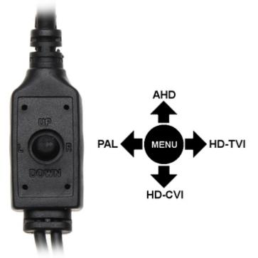
Configuration 1) Move the joystick in the correct direction
