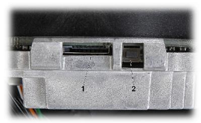
1. Memory card slot 2. RESET button Mounting side view:
