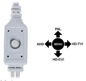
Configuration 1) Move the joystick in the correct direction 2) Turn on the power In the kit:
