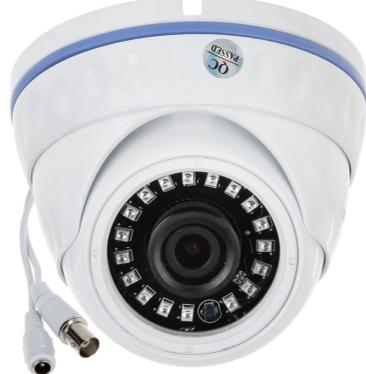
Megapixel camera with 1/3" CMOS sensor and AHD / HD-CVI / HD-TVI / PAL.
