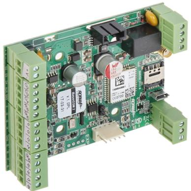
The device dedicated for integration with alarm control panels, controllers, relays, etc. via binary inputs and outputs. The terminal is equipped with analog inputs for cooperation with e.g. temperature sensor, and with LogicProcessor providing advanced logic functions allowing for the implementation of simple home automation systems. In combination with an embedded GSM module allowing for remote control, notification, the device is suitable for very wide range of applications.
