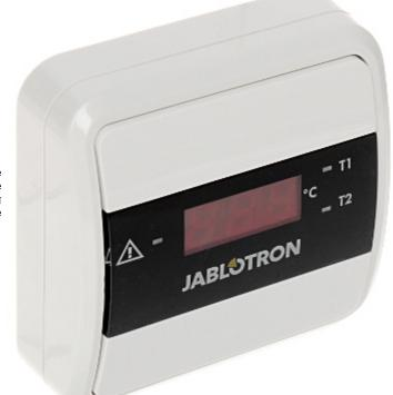
The TM-201A multi-function thermometer enables temperature measurement with using up to 2 sensors CP-201T-NW (available separately). The device can work as: thermometer indicating exceeding the preset temperature, monostable thermostat, bistable thermostat, differential thermostat.
