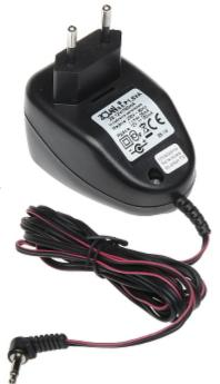
Attention! If the power adaptor is using for continuous work (24H) the rated current of the adaptor should be less than 80% of the maximal current.
