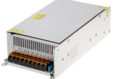
Power adaptor with three pairs of output terminals. Attention! If the power adaptor is using for continuous work (24H) the rated current of the adaptor should be less than 80% of the maximal current. Attention! Three -V adapter terminals are physically
