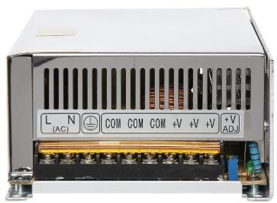
L - Live wire (230V) N - Neutral wire GND - Grounding COM - DC "-" output +V - DC "+" outputs ADJ - Output voltage adjustment Input voltage switch:
