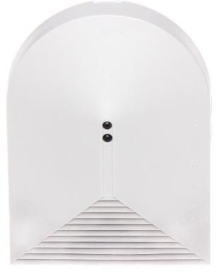
Sensor signals an alarm on registering a low-frequency tone (impact sound), followed by a high-frequency tone (sound of broken glass). The sensor starts to analyze a high-frequency channel after receiving the low-frequency sound wave, caused by the impact.
