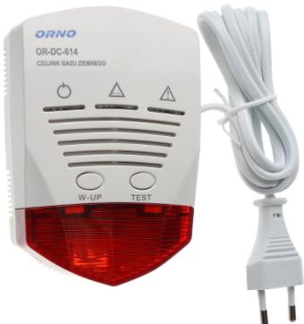
The OR-DC-614 is a device designed for continuous monitoring of natural gas concentration in the air. This device should be installed in a closed indoor rooms with high risk of gas exposure. Gas concentration above the threshold level triggers visual and audible alarm signals. The device should be mounted in high position, just under the ceiling.
