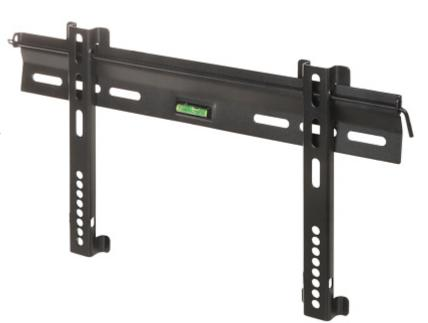
The BS-106S mount is intended for hanging a TV or LCD / OLED monitor on the wall. The bracket is equipped with built-in bubble level tool, which enables precise and quick installation. It should be mounted on the surface, which construction has to carry the required load, including a wide margin of safety. Maximal load capacity is 45 kg.
