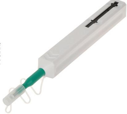
The WUN-XK25 tool is used to clean the end face of the ferrule in fiber optic connectors. A special fabric removes any contaminants, and its antistatic properties prevent dust from settling again. The product is suitable both for cleaning connectors in adapters mounted individually and mounted in patch panels.
