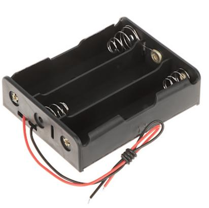
A holder for 18650 cells solves the problem of connecting them in many electronic projects (eliminates the need to weld into a package or solder cells). The holder has metal contacts and wires with removed insulation at their ends, which ensure a secure connection between the battery and the target device. The connections made in the holder are serial.
