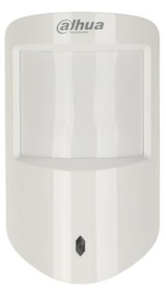
Wireless motion detector, which is designed to detect the moving intruder within the system protected area. With a combination of PIR and MW detection was reached high immunity to false alarms. Thanks to pet immunity, the ARD2231-W2(868) can provide protection even when small pets are moving around during surveillance.
