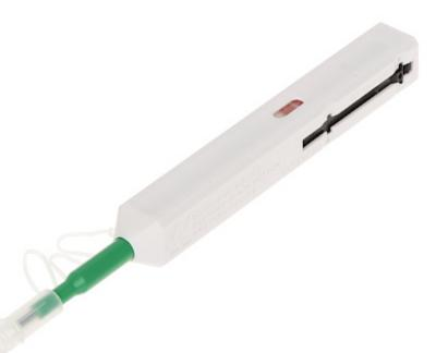
The WUN-014 tool is used to clean the end face of the ferrule in fiber optic connectors. A special fabric removes any contaminants, and its antistatic properties prevent dust from settling again. The product is suitable both for cleaning connectors in adapters mounted individually and mounted in patch panels.
