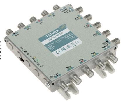
The SD-515 splitter is used in multiswitch systems to distribute a signal from multiswitch bus. Additionally, the splitter also distributes terrestrial TV signals. The splitter is equipped with DC-transition switch that in "ON" position passes DC voltage through "H" paths to both branches. In "OFF" position it runs voltage to one path only.
