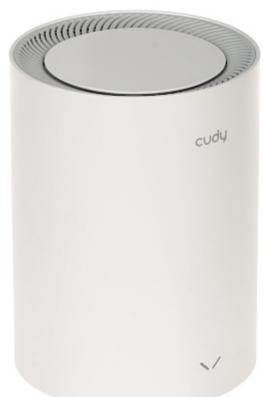
The CUDY-M1800 access point broadcasts 2 separate wireless networks in the 5 GHz band with speed 1201 Mb/s and in the 2.4 GHz band with speed 574 Mb/s. Simple tasks such as sending e-mails or web browsing can be handled by the 2.4 GHz band while bandwidth intensive tasks like online gaming or HD video streaming can be processed by the 5 GHz band – all at the same time.
