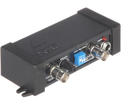
The VCA-1/2000 is designed to amplification of the video signal transmitted via coaxial cable, what enables video transmission up to 2000 m distance. The control knob perform both gain adjustment and correction of frequency response functions. Together with increase of gain, the correction is deeper. **The amplifier must be used at the end of the transmission line (close to the monitor).**
