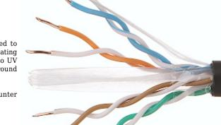
The UTP/K6/305M/PE twisted-pair cable is designed to professional applications of installation. The outer coating is made from polyethylene (PE) which is resistant to UV radiation and humidity. The cable is suitable for ground installations, in cable ducts.
