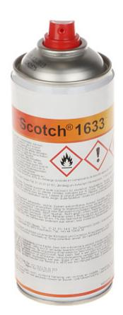
The SCOTCH-1633/400 preparation is a multifunctional rust-removing aerosol in the form of oil with the addition of molybdenum disulphide. This agent removes rust, and protects the material against moisture and re-oxidation. The base component of the preparation is mineral oil, which allows it to be successfully used as a lubricant.
