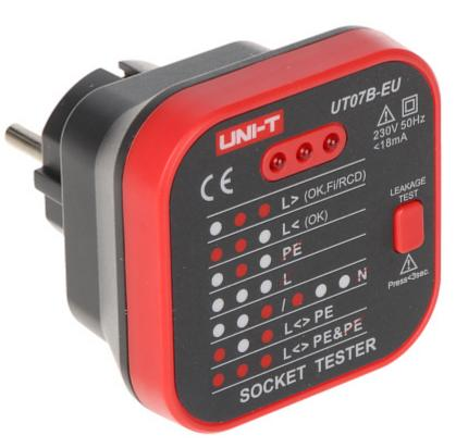
The UT-07B-EU tester indicates the correctness of the L, N, PE wiring in the electrical socket. In addition, it has the function of testing the efficiency of the operation of RCD residual current devices.
