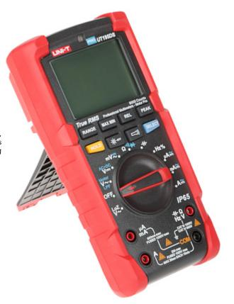
The UT-195DS is a universal digital meter used to measure: voltage, current, resistance, capacitance, frequency, and checking the correctness of diodes operation. The meter has the function of automatic change of measuring ranges, as well as the relative measurement mode.
