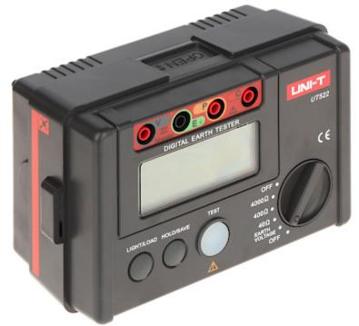
The UT-522 meter allows to measure: grounding resistance of power installations, grounding resistance of devices, resistance of lightning protection systems, etc. The design of the device allows for a complete, accurate measurement of the grounding resistance using 3 leads and a simple, approximate measurement using 2 leads.
