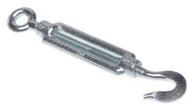
Turnbuckles are used to tightening and regulations of the lines. Tension adjustment is possible by screwing oppositely directed threads located within the body.
