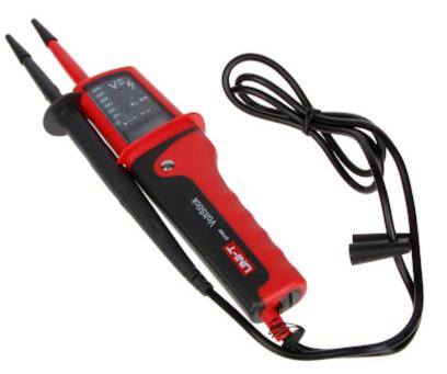
The UT-15C meter allows to measure AC, DC voltages in the range 12 ... 690V. The measurement is carried out automatically when the probes come into contact with the measuring points. The device automatically selects the appropriate measuring range and informs the user about it using LEDs located above the display.
