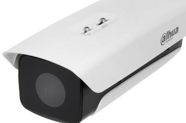
The PFH610V-H-POE-V2 housing is designed for cameras powered according to the PoE 802.3af/at standard. The half open housing equipped with heaters with thermostat and cooler fan.
