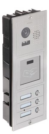
Video Doorphone is mounted in a flush-mounted housing. Surface mounting is possible with the D600B3 cover. Built-in RFID reader allows to control the electric strike using key fobs, proximity cards and tags functioning in the Unique EM 125kHz standard. The S603A-2 is designed to cooperation with video doorphones and panels working in analog VIDOS system.
