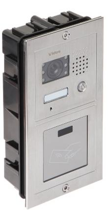
Video Doorphone is mounted in a flush-mounted housing. Surface mounting is possible with the D600B3 cover. Built-in RFID reader allows to control the electric strike using key fobs, proximity cards and tags functioning in the Unique EM 125kHz standard.
