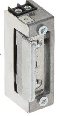
The electric strike of R4-24.13 type is designed for door and gates made from metal profiles, to work together with ratchet-latch or ratchet type door lock. It operates reversibly - it is open when power is off.
