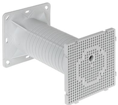
Mounting desk for installing electrical devices (eg outdoor lights, motion sensors, etc.) on thermally insulated buildings facades with a thickness from 50 to 200 mm. The robust construction. Elimination of thermal bridging. Before installing, it is necessary to cut the carrier including the enclosed insulation to the required length according to the thickness of the insulating layer.
