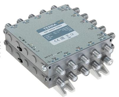
The SD-904 splitter is used in multiswitch systems to distribute a signal from multiswitch bus. Additionally, the splitter also distributes terrestrial TV signals. The splitter is equipped with DC-transition switch that in "ON" position passes DC voltage through "H" paths to both branches. In "OFF" position it runs voltage to one path only.
