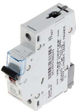
Thermal-magnetic circuit breaker with B-type curve and 10A rated current. The LE-403355 circuit breaker is compatible to DIN TS-35 rail mounting system. Circuit breakers with B-type breaking curve are designed to protection against short-circuits and overloads of the lighting, control circuits and outlets.
