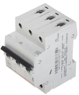
Thermal-magnetic circuit breaker with B-type curve and 20A rated current. The LE-419170 circuit breaker is compatible to DIN TS-35 rail mounting system.
