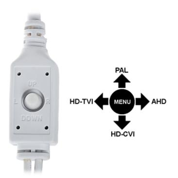
Configuration 1) Move the joystick in the correct direction 2) Turn on the power Option 2:
