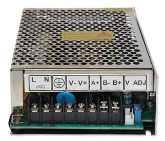
Live wire (230V) Neutral wire Grounding DC "-" output DC "+" output A+ Not connected B- (+) battery output B+ (-) battery output ADJ - Output voltage adjustment
