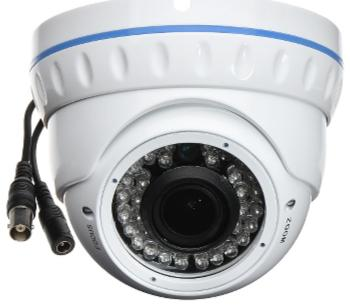
Megapixel camera with 1/2.7" OmniVision OV2710 CMOS sensor and HD-TVI (High Definition Transport Video Interface). The HD-TVI interface allows to transmission of analog video signal via coaxial cable at resolutions up to 1080p. It enables the transmission of HD resolution images for even 500 m distance with keeping the low costs of the installation. During transmission there are no delays and is maintained the original, high quality image.
